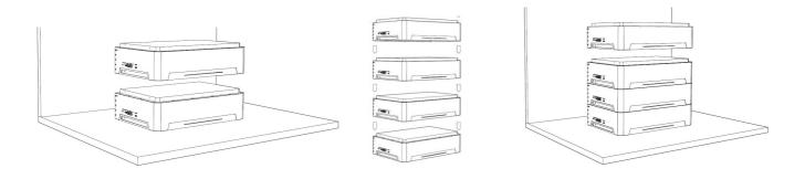
Installers should pay attention to the direction during installation. They shall be installed vertically and shall not be tilted.
